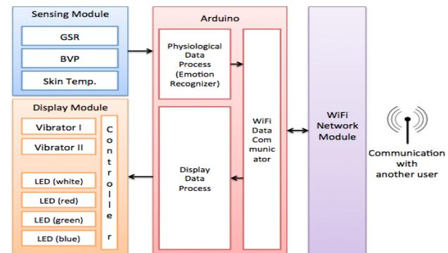
**Figure 2.** A System Block Diagram of Empa Talk
