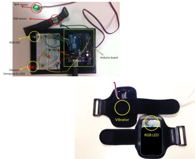
**Figure 3.** Empa Talk prototype device (up) and Armband with Vibrator and RGB LED (down)
