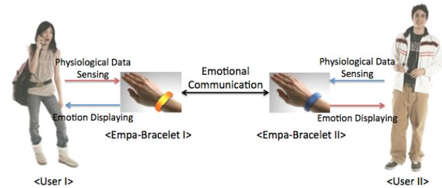
**Figure 1.** The concept of Empa Talk communication
