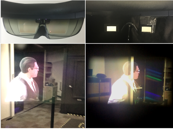
Fig. 4. View conditions and captured photos for each condition: (left) unrestricted, (right) restricted. The augmented field of view is 30^\circ \times 17^\circ . The images here show only a small peripheral area because of photographing constraints. The peripheral FOV perceived through the HoloLens is much larger.
